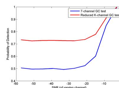
Figure : (Left) Empirical probability of detection ( $P_d$ ) as a function of the varying SNR on channel 7. (Right)  $P_d$  as a function of the varying SNR on channels 4, 5, 6 and 7. The red lines show results from the full 7-channel GC detector, blue lines show results with censoring prior to the GC detector.  $P_f$  is held constant at 0.1.
