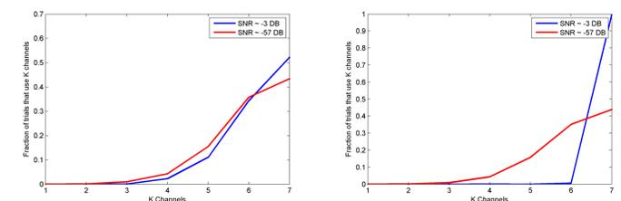
Figure : Sample distributions of  $K$ , the number of channels used in the second (fusion) stage. (Left) Representative of the experiment with one channel of varying SNR. (Right) Representative of the experiment with 4 varying channels.
